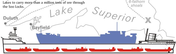
The *Fitz* was 729 feet in length--over 300 feet longer than an LST (shown in blue atop the Ore Freighter). It would take over six LCTs (shown in red) to equal the length of the *Edmund Fitzgerald*.
